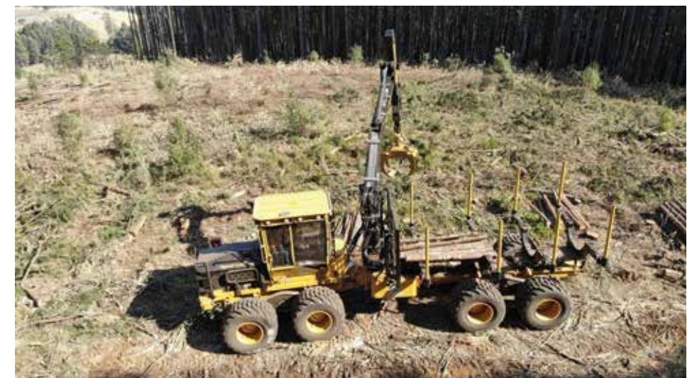
Tigercat forwarder collects harvested timber in-field and hauls it to the roadside depot.
