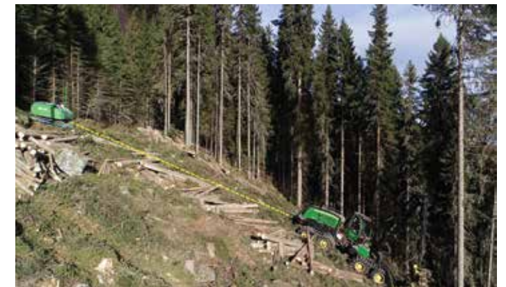
An example of a winch-assisted machine, in this case a John Deere 1470 attached to a T-winch from Ecoforst (cable line is schematic).
