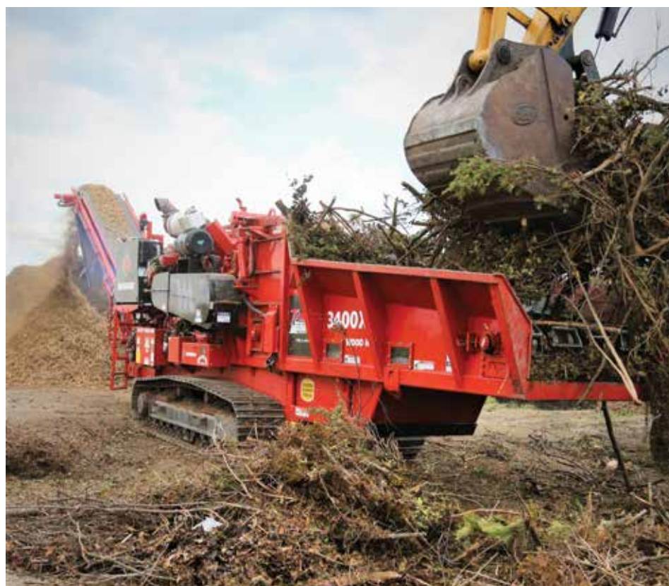
Morbark grinders are designed to reduce all kinds of wood and tree waste for multiple uses.
