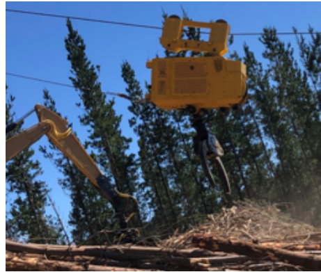
Alpine Drop Carriage suspended from the Top Truck.
