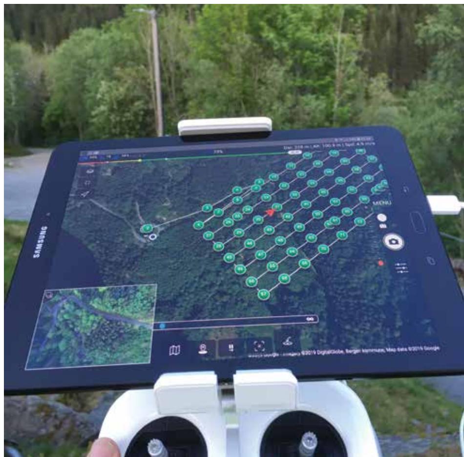
Correct planning of a drone survey mission is essential in generating data of a useable quality and this is an area that needs further cooperation between forest planners and drone operators
