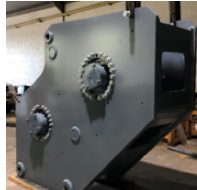
This massive 600m double drum live skyline winch-set will be mounted at the rear of the excavator, replacing the counterweight.
