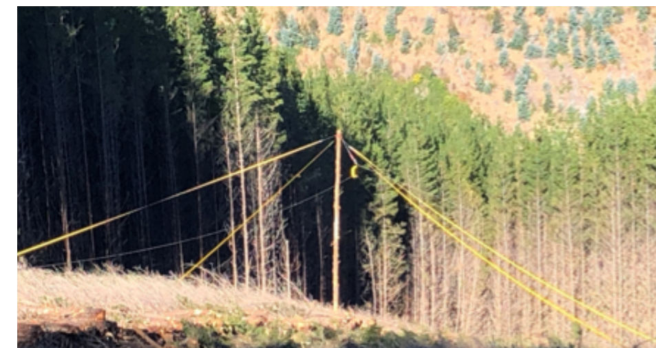
An Intermediate support being rigged up for an Alpine Drop Carriage
