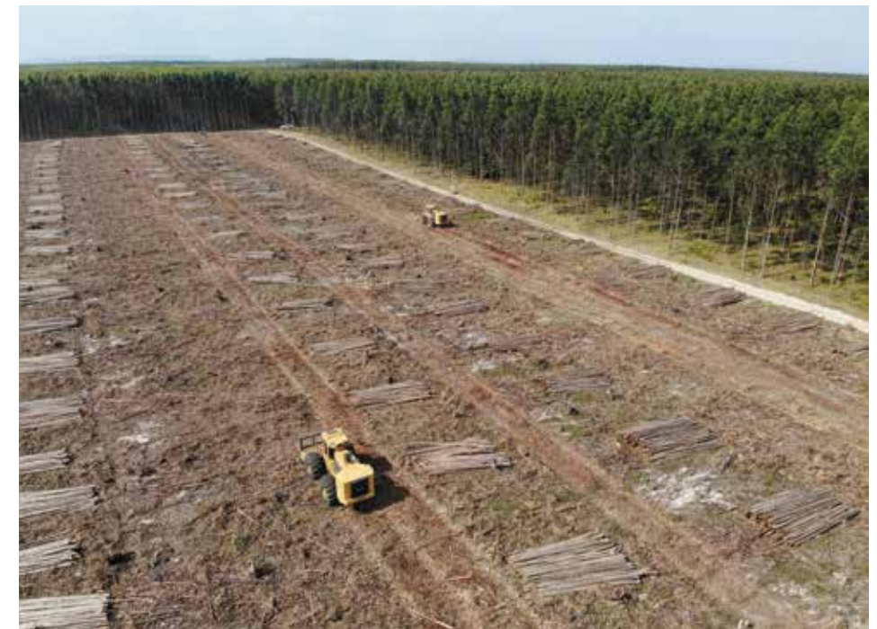
Tigercat M726G mulchers reducing slash on extraction routes in Zululand.
